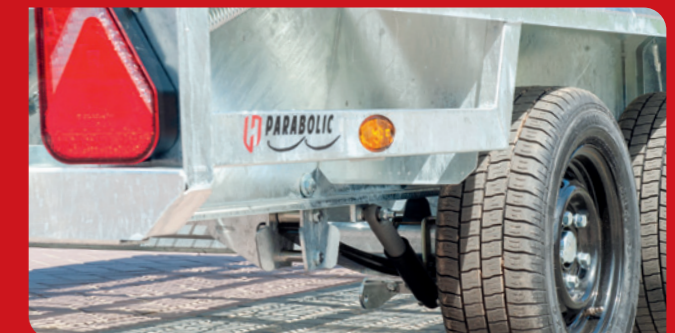
Parabelfederung Parabolic suspension
